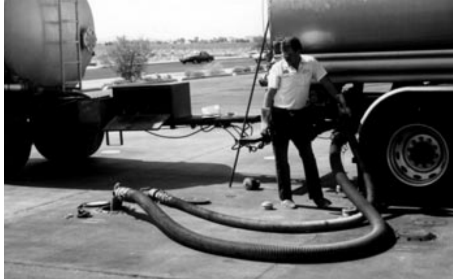
Operator vigilance during delivery is critical to spill prevention.
