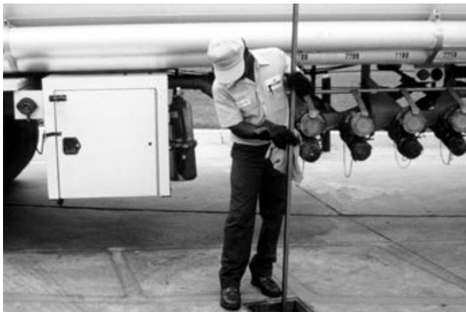
Determining the ullage in a tank prior to delivery is critical to preventing overflow incidents.
